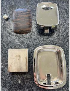
Three of the pieces are bright nickel plated: the knob and the two shell pieces. The metal insert is wood-grained to match the rest of the interior trim pieces. On the back of the shell is the manufacturer's logo: Grand Rapids Metalcraft.
