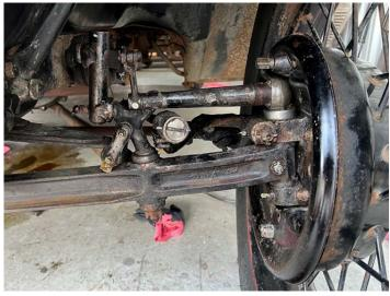
Finer Points continued from page 2 - Next, we can take a look at one of the wheels. Obviously, the tire had to be replaced to make the car safe to drive. Everything else is original including the valve stem, short lug nuts, and early hub cap. The red centering line on the tire is how it would have come from the factory.
