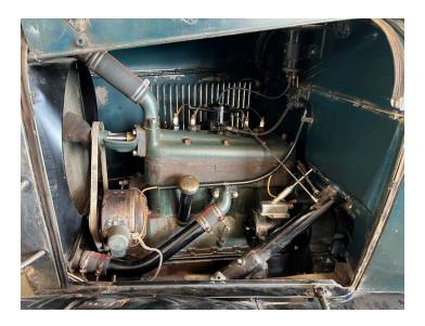
Now, let's move to the passenger side of the engine compartment. From this view, you can see the solid front motor mount at the front cross member. Additionally, the original tail pipe and the engine pan are both visible. Unlike later styles, the front of the engine pans attach to the front cross member.
